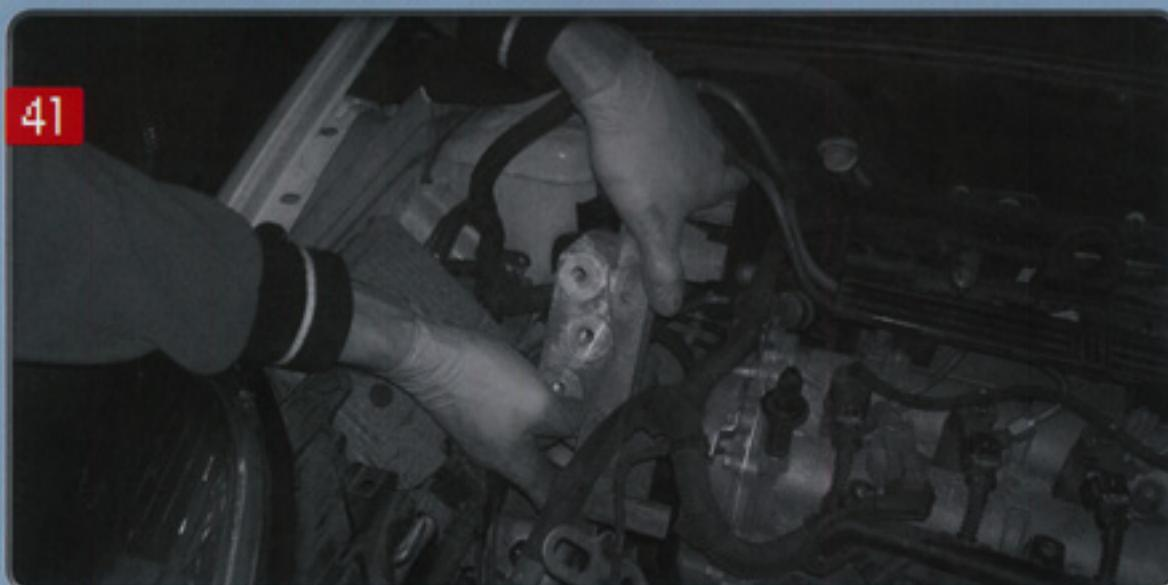
DOPO AVER TOLTO I SUI FISSAGGI, ESTRARRE DAL SUO ALLOGGIAMENTO LA PIASTRA DEL SUPPORTO MOTORE SUPERIORE DESTRO.
